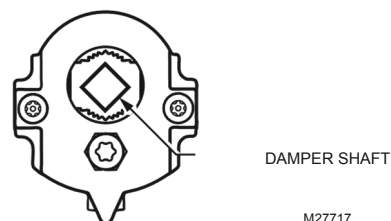
Fig. 6. Proper mounting to square damper shaft.
